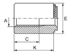
Female thread A = M4Height K = 22Min distance to edge = 4.0Outer diameter E = 8Plate thickness = from 2.4Recommended bore diameter +0.05 = 5.00Thread length = 8.0
